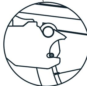
4. Push the handlebars on the Infinity at an angle upwards while leaning slightly backwards to lift the wheelchair's castors from the ground and lock the Infinity against the lower dock (G). When Infinity is connected to the lower docking point, a clicking sound is heard.
