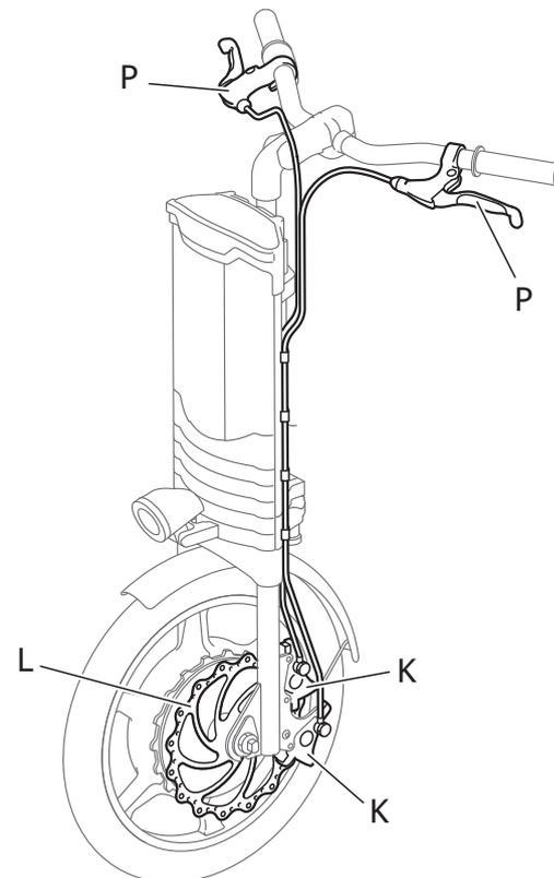
It is extremely important that the distance between the brake lever and the steering lever is not less than 15 mm when the brake lever is retracted as far as possible. Otherwise the braking capacity will not be sufficient
