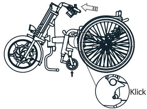
5. First push the locking handle (D) forward to release it. Then slide it back to lock the Infinity to the adapter bar. The support legs (J) are now raised.
