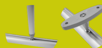
Anchoring on profile rail: possible along the whole length by means of square nut; for adjustable ceiling mount RVS/DS or with ceiling bracket RVS/DH. Max. spacing: 2 m.
